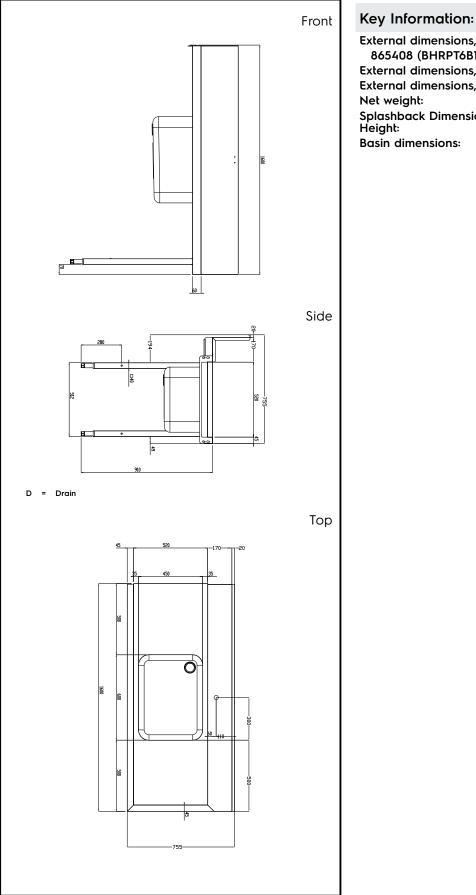
External dimensions, Width: 865408 (BHRPT6B16R) 1600 mm External dimensions, Depth: 755 mm External dimensions, Height: 1170 mm 28 kg Splashback Dimensions, 260 mm
